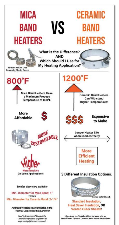
between pieces of mica, there is better heat transfer from the ribbon to the exterior surfaces of the heater. Also, in general, mica band heaters will have less unheated area than a ceramic band heater, especially in smaller band heaters.
