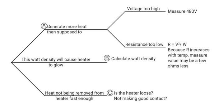
The first thing I suspected was watt density. Watt density is calculated as follows:
