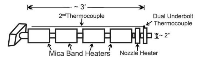
In this particular example, heater wires are stainless steel overbraid. Thermocouple wires are inside the hose. Probes are wrapped in aluminum foil before being inserted into a mold that is the size of small car. Sometimes, the thermocouple is damaged while being inserted into the mold. The customer's thought was to measure the resistance of the thermocouple after insertion as an indication of whether the thermocouple was good.
